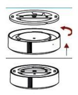
Ease of Replacement: Just twist & fit the light onto the Bracket
