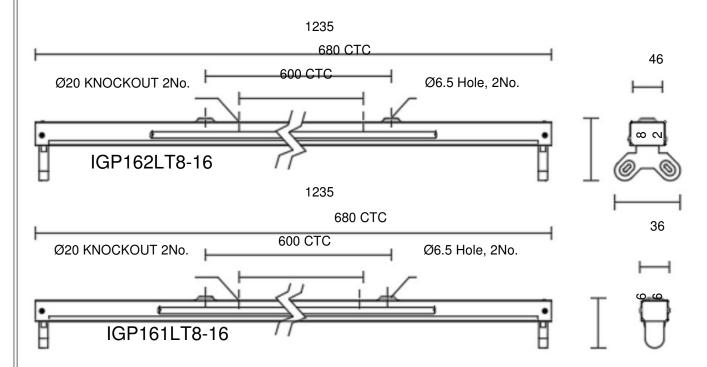
DIMENSIONS SHOWN ARE FOR INSTALLATION REFERENCES ONLY AND WILL BE VARYING ACCORDING TO THE MFG. PROCESSES.
