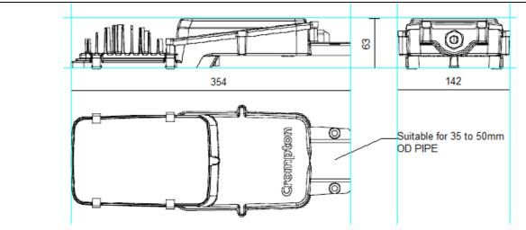
DIMENSIONS SHOWN ARE FOR INSTALLATION REFERENCES ONLY AND WILL HAVE TOLERANCE ±3mm UNLESS OTHERWISE SPCIFIED
